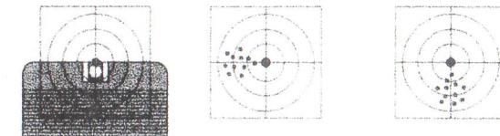
□ To aim the left, turn with a right-angled screwdriver the right screw on the rear sight rightward. It would be deflected to the left if rotate it leftward.
