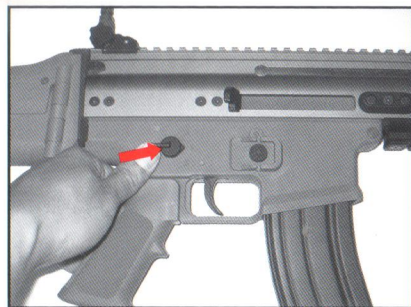
左側位置 The selector button on left side for left hand shooter.
